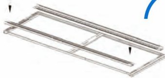
1A. Assemble mounting rail(only width 600mm). (Screw M6x12 & nuts).
